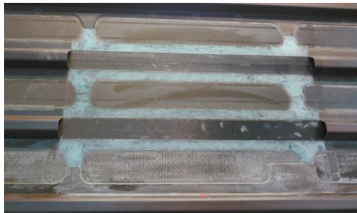
Figure 3-2. Inside of a fuselage side shell showing the partly removed stringers.
